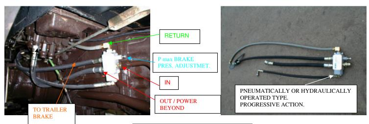
PNEUMATICALLY OR HYDRAULICALLY OPERATED TYPE. PROGRESSIVE ACTION.
